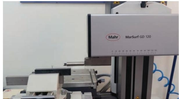
Fig. 2. A sample photograph of the roughness measurement
