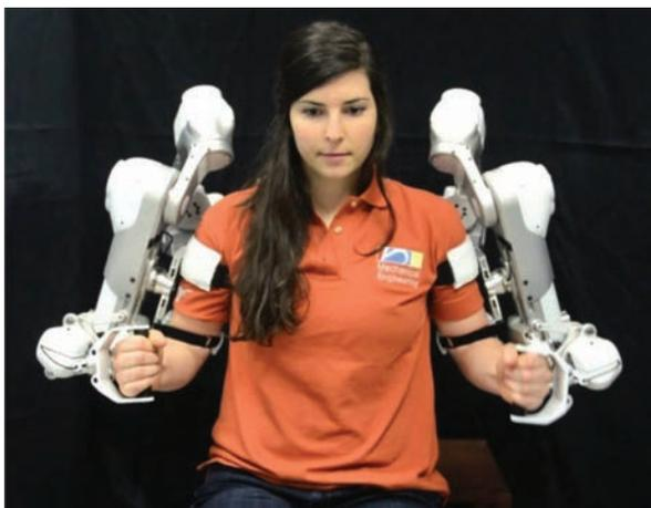
Fig. 2. A photo of the rehabilitation robot Harmony
