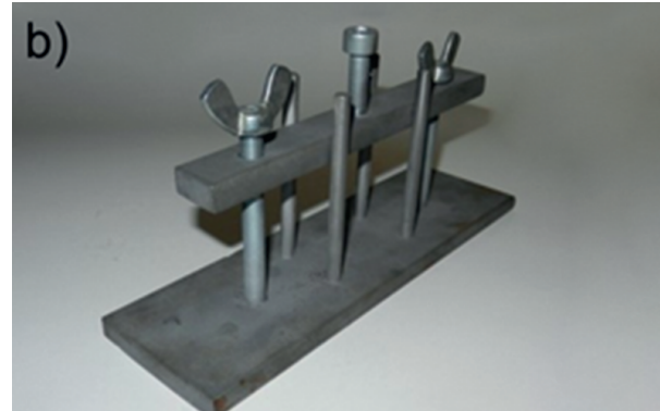
Fig. 9. Prototype devices: a) to form sample elements, b) for stabilizing glued samples
