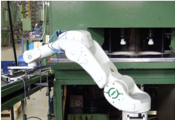
Fig. 8. Installation of the system on the tapered roller bearings' production line
