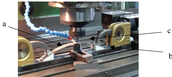
Fig. 4. Preparation of the sample measurement area: a) sample patch; b) grip; c) end mill
