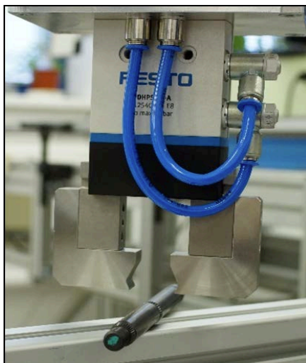
Fig. 7. Finger gripper – two finger version and its parameters [10]
