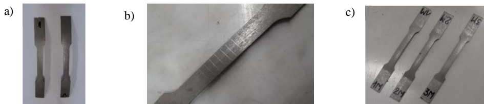
Fig. 5. Test samples a) after milling, b) after tracking, c) with flattened ends
