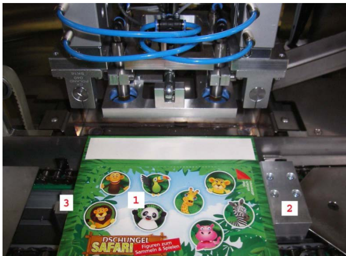
Fig. 5. Principle of the box positioning on the chain conveyor
