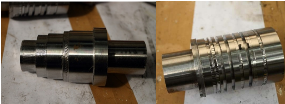
Fig. 3. Marks of unstable machining: (a) in longitudinal turning b) in cutting
