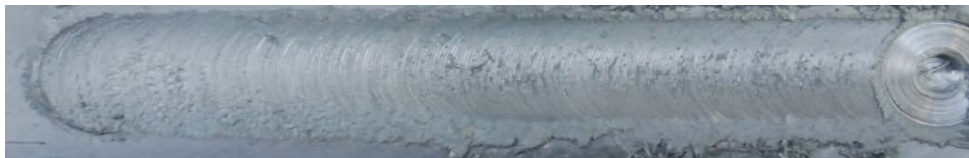
Fig. 10. The view of the weld surface
