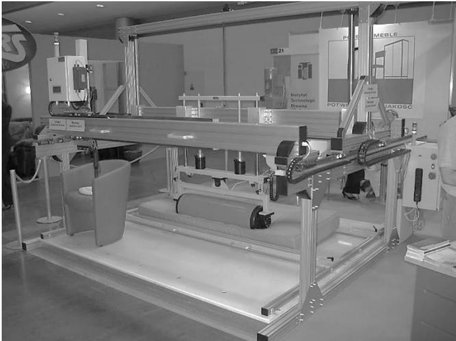
Fig. 1. a) Device for testing the rotary bases of office chairs and for rotation test of chair according to p. 7.3.3 and p. 7.3.5 of the PN-EN 1335-3:2009 standard, type **BK-EN 1335-3**, b) Device for impact testing the furniture, type **MU-M/D**, c) Device for testing the endurance and hardness of bed frames according to PN-EN 1957:2002 standard 5, 6
