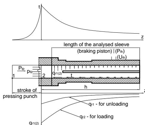
Fig. 2. Scheme of loads within the sleeve
