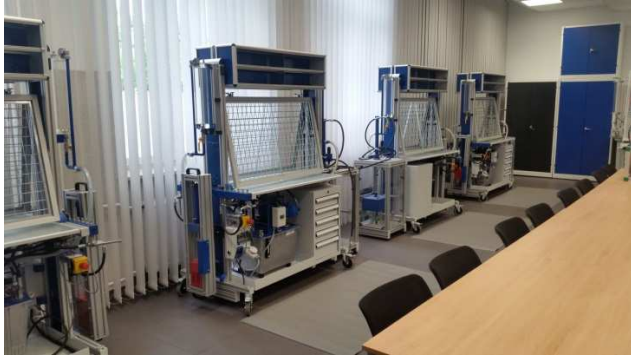
Fig. 1. Teaching and research stations for mobile hydrotronics of robot drives from Bosch Rexroth at the laboratory of hydrotronics and automatic control of mobile robot drives
