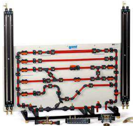
Fig. 5. Station for determining losses in hydraulic piping installation [1]
