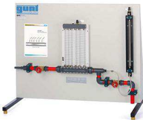
Fig. 4. Station for determining the impact of changes in the size of cross-section of installation on the potential and kinetic energy of liquid [1]
