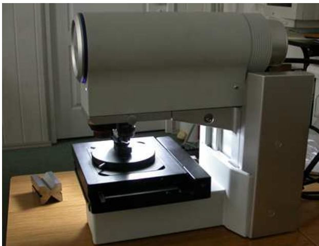
Fig. 1. Image of an optical-digital microscope for contactless investigation
