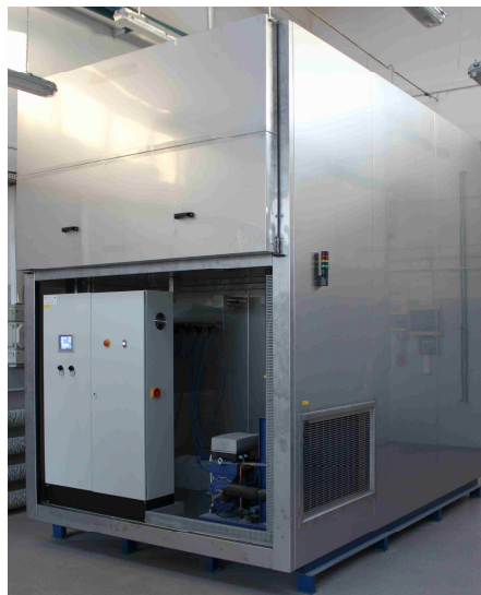
Fig. 5. View the climatic testing stand, produced by ITeE – PIB
