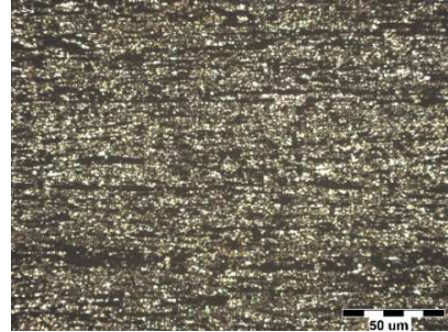
Fig. 3. Surface of X2CrNiN23-4 steel annealed at 485°C for 30 min. and cooling down on air after corrosion tests in boiling HNO 3 for time = 48 h
