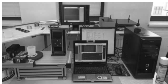
Fig. 8. The test stand to scan the side surface of products
