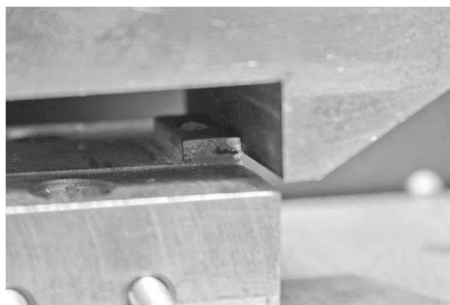
Fig 6. The position of the impactor with regard to the sample at the time of applying the load
