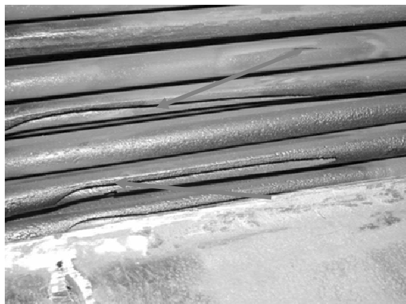
Fig. 1. An image of the perforations of tubes of a heater located opposite the piping feeding steam to the heat exchanger [12]
