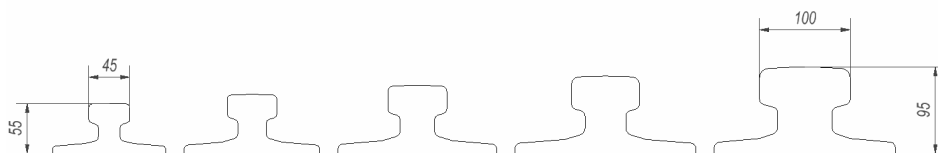
Fig. 4. Crane rail dimensions [7]
