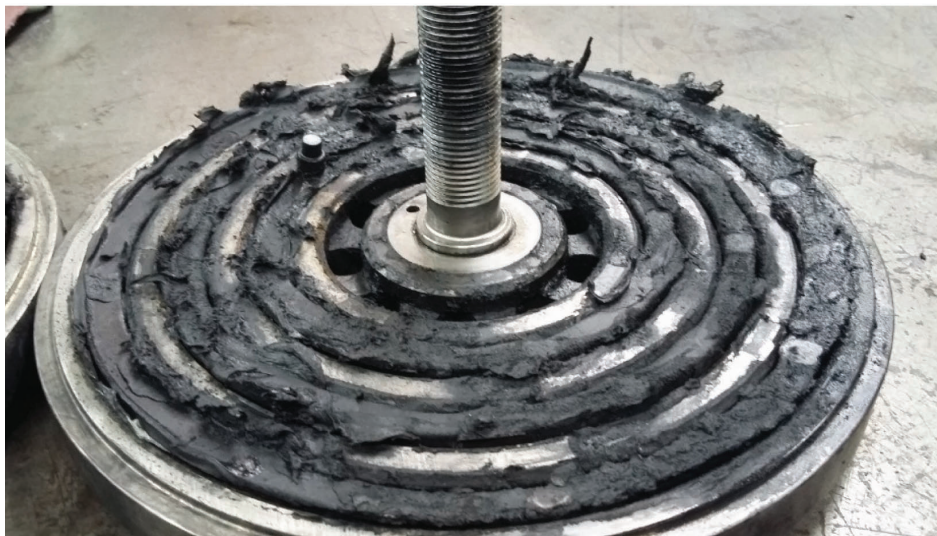
Fig. 6. A heavily contaminated discharge valve seat
