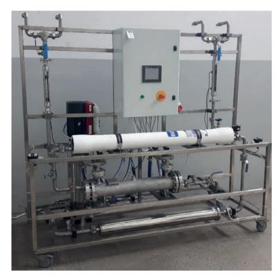
Fig. 7. Prototype membrane ultrafiltration plant Source: Authors.
