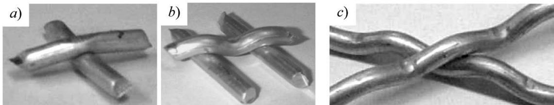
Fig. 4. Modelling of interaction (a) and deflection (b) of the wire turns by discrete samples, and by wire package samples (c)
