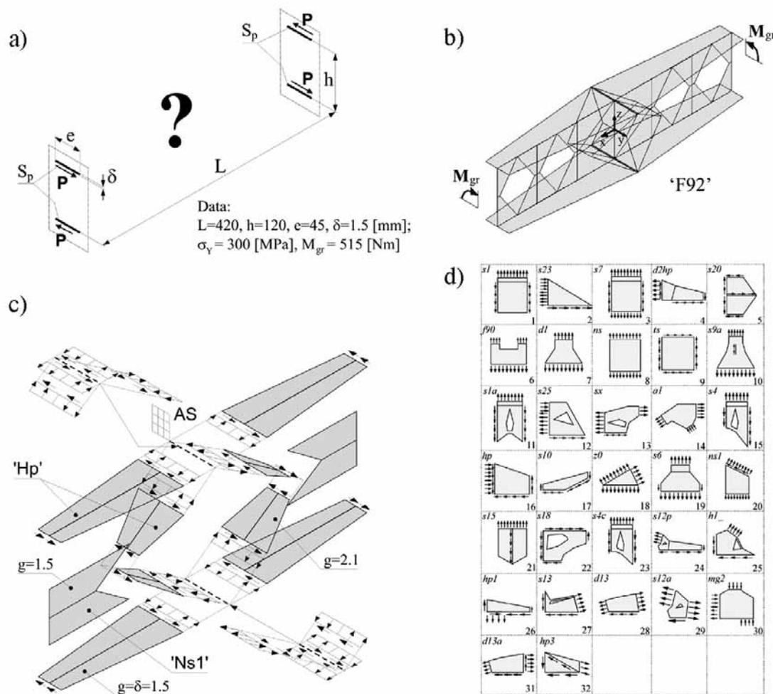
Fig. 1. Formulation and solution of design problem [3]: a) illustrative presentation of boundary conditions and problem formulation; b) statically admissible solution, complex spatial field that determines the structure; c) allocation of component library fields and interactions between them in the complex field; d) library of particular solutions from SADSfAM software package
