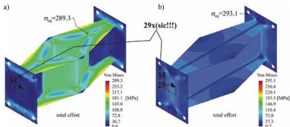
Fig. 10. Comparison of distributions of total equivalent stress in the model designed by SADSF method and the model of simple I-section
