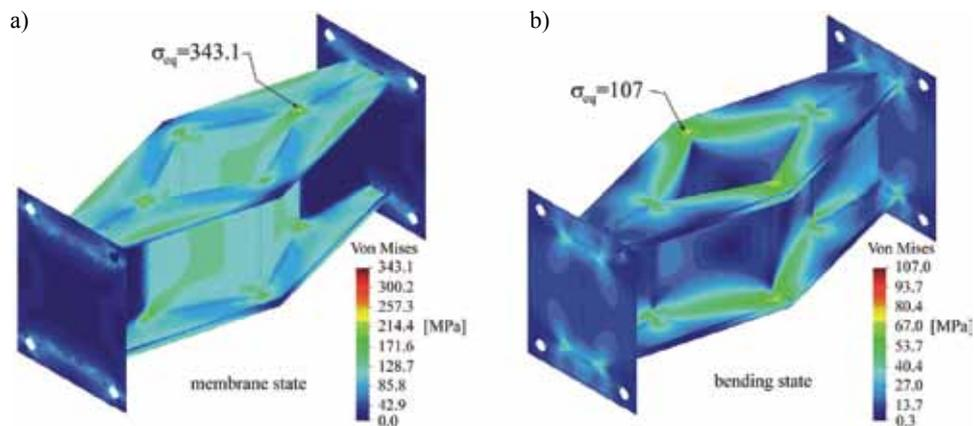
Fig. 9. Distributions of equivalent stress in the model with edge stiffeners on flanges shown in Fig. 7b
