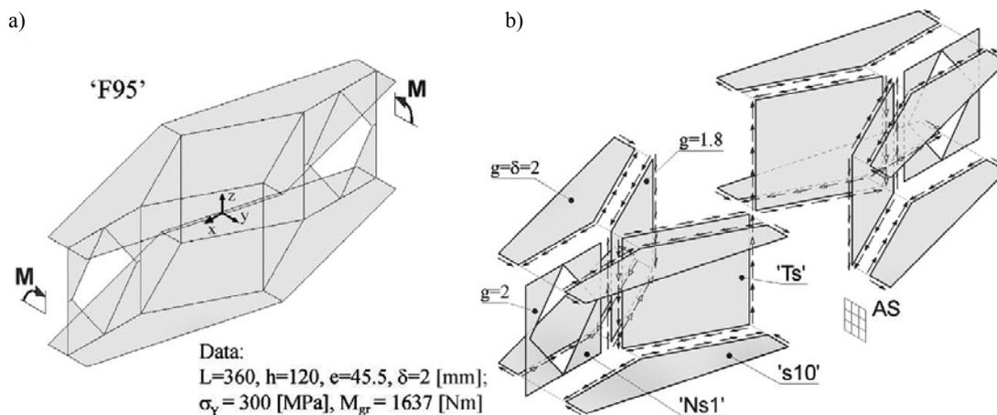
**Fig. 2. Another example of solution to the problem from Fig. 1a [3]: a) contours of the model determined based on statically admissible stress field; b) spatial allocation and interactions between component library fields in the complex field**
