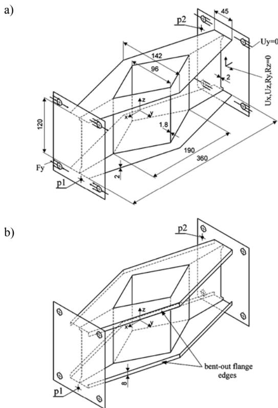
**Fig. 7.** Shape and dimensions, and boundary conditions assumed for FEM calculations of analysed models based on solution 'F95' from Fig. 2a [1]: a) model corresponding exactly to SADSf solution; b) model with edge stiffeners
