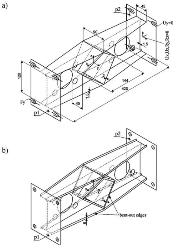
**Fig. 3. Shape, dimensions and boundary conditions assumed for FEM calculations of analysed models based on solution from Fig. 1b [1]: a) model corresponding exactly to SADS solution; b) model with introduced modifications – edge stiffeners on flanges and oblique elements**
