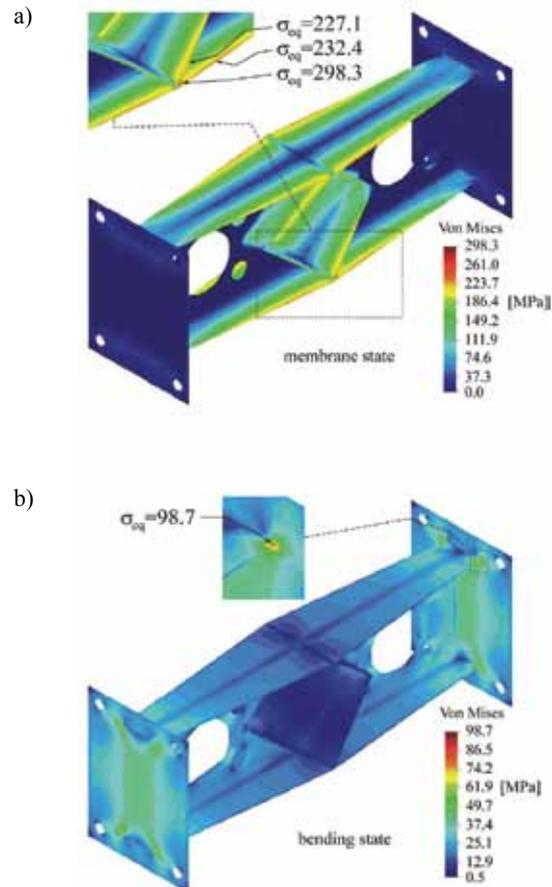
**Fig. 4. Distributions of equivalent stresses in model from Fig. 3a calculated according to Huber-Mises yield criterion**
