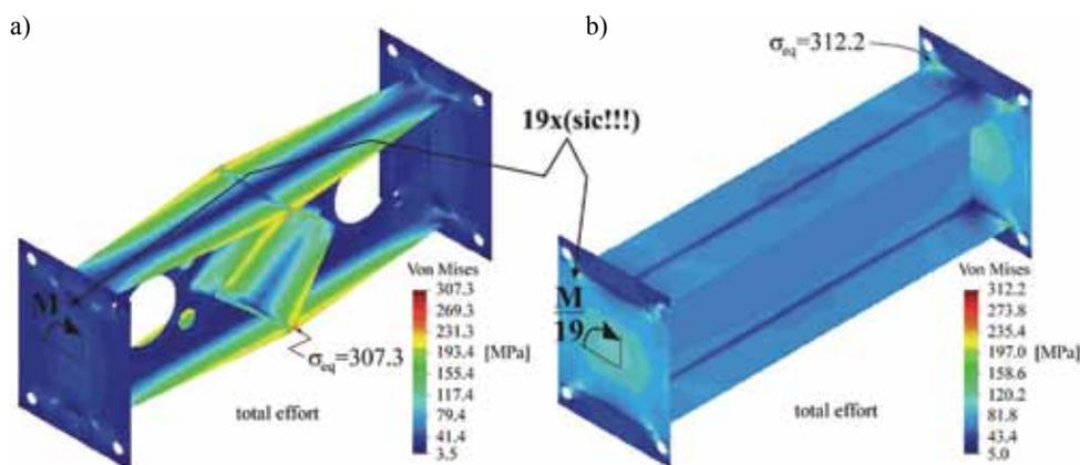
Fig. 6. Exemplary comparison between distributions of total equivalent stress in the model designed by SADSf method and the model of simple I-section
