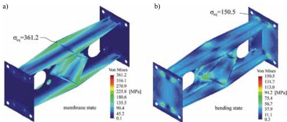
Fig. 5. Distributions of equivalent stresses obtained for the model of torsion-loaded shell with edge stiffeners on flanges and oblique elements shown in Fig. 3b (calculated according to Huber-Mises yield criterion)
