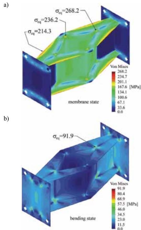
**Fig. 8.** Distributions of equivalent stress in the model from Fig. 7a calculated according to Huber-Mises yield criterion
